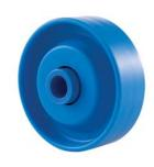
Our UNI-FLEX™ standard is 49mm dia heavy duty zinc plated steel suitable for all flat based loads. We can also offer a 48mm dia plastic skatewheel for lighter duty applications if required. Please note that the conveyor load capacity is reduced to 80 kg′s per linear metre with plastic skate wheels.
